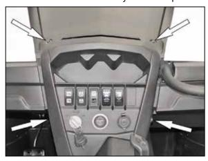
23. Reinstall the center dash and secure with the factory hardware.
