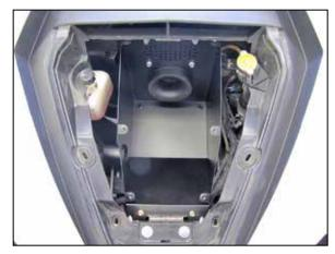
21. Set the air box into position and secure it to the K&N® bracket with the hardware provided. Secure the front of the box with the factory air filter housing bolts removed earlier.
