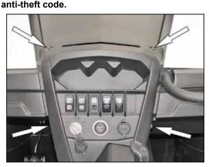
2. Remove the two bolts and two plastic clips securing the center dash, then remove the center dash and set aside to gain access to the intake system.
