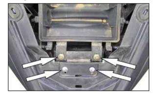
6. Remove the two rivets shown securing the upper body work to the chassis and then remove the two bolts securing the lower air filter housing to the chassis.
