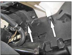
9. Remove the four bolts securing the front body work.
