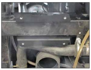
18. Install the K&N® air filter box mount over the frame cross member.
