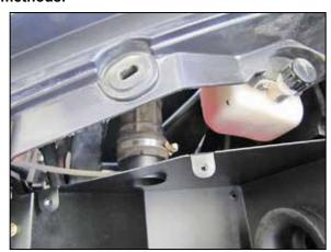
22. Connect the fresh air intake hose to the air filter box and secure with the factory hose clamp.
