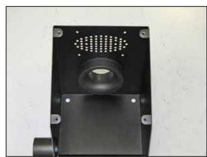
19. Install the radius adapter into the air filter box and secure with the provided hardware.
