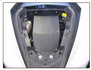
25. Install the K&N® air box lid and secure with the provided hardware.
