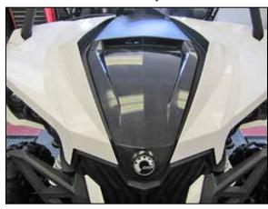
4. Remove the hood panel to access the air filter housing.
