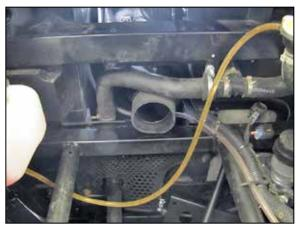
16. Install the provided hump coupler (087121) onto the K&N® intake tube and secure with the provided hose clamp.
