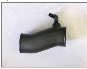
14. Install the provided 90° fitting into the K&N® intake tube.
