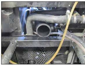
15. Install the K&N® intake tube into the coupler hose at the throttle body, the vent fitting should be on the driver's side of the vehicle and on the front of the tube. Connect the crank case vent hose to the fitting installed into the K&N® intake tube and secure with the factory spring clamp.
